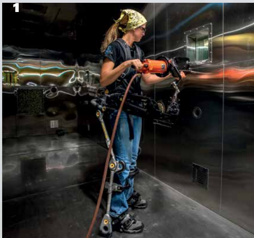
1. Lockheed Martin's unpowered FORTIS exoskeleton takes the weight of a load like a heavy hand tool off operators and is currently under test with the US Navy.
